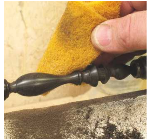
▲ Pic.30 After sanding through the grits, for safety finish the work with a Nyweb pad, which tends not to grab the spinning work; this one is the equivalent of 0000 wire wool
